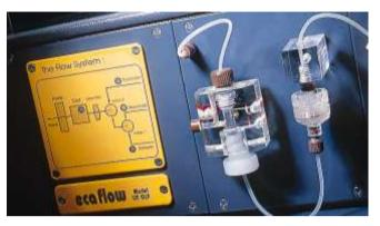
The compact flow system is controlled by the control unit and operates fully automatically. It contains computer controlled electromagnetic valves for switching either to the sample solution or to an electrolyte solution or to a standard solution for the standard addition. The solutions are driven by a peristaltic pump. The heart of the system is the patented compact electrochemical cell.
