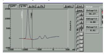
Moreover, if appropriate, the system enables to measure in the classical voltammetric mode by making use of any electrode system e.g. hanging mercury drop electrode, wall-jet electrode, rotating disk electrode of various provenience.
